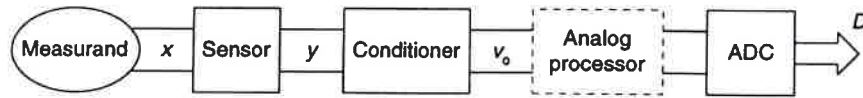
FIGURE 1.7 General structure of a system that obtains a digital code D from a measurand x .
