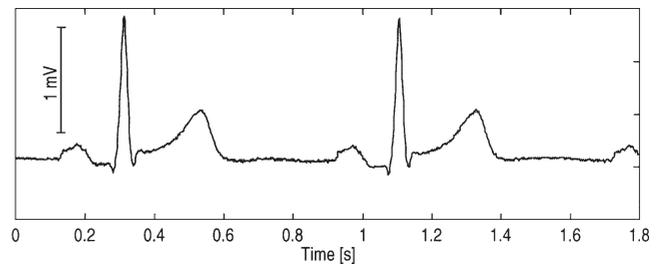
Fig. 4. ECG signal acquired by the proposed amplifier. No other signal processing except for a bandwidth limitation to 128 Hz was performed.
