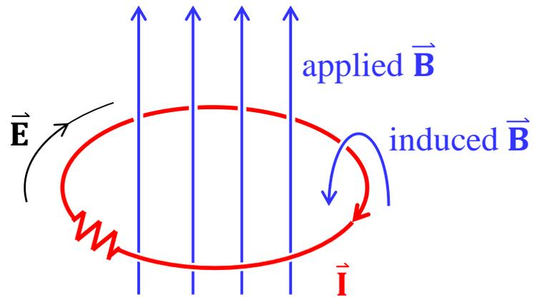
**Fig 9.3** Induced emf due to a stationary loop in a time varying B field.
