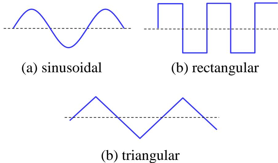
**Fig 9.1** Various type of time-varying current
