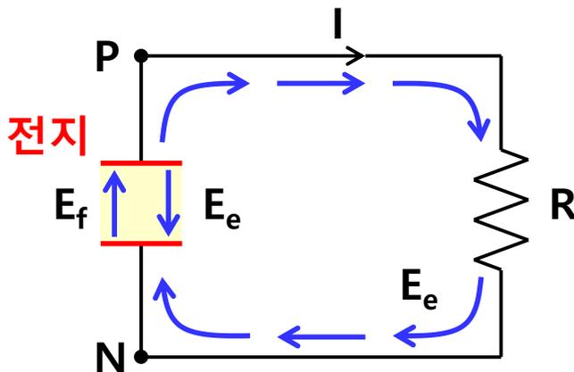
**Fig 9.2** Circuit showing emf-producing field  $E_f$  and electrostatic field  $E_e$ .
