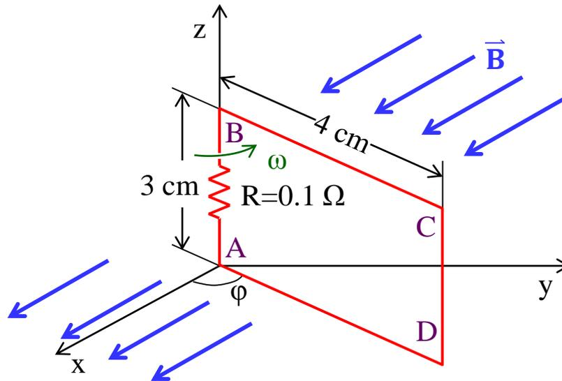
**Figure 9.7** For example 9.2; polarity is for increasing emf.
