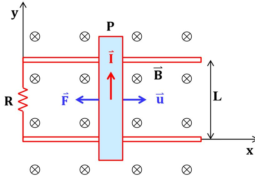
**Fig 9.5** Induced emf due to a moving loop in a static B field.
