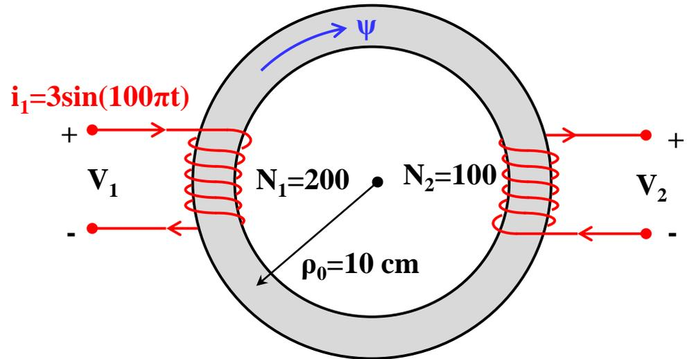
**Fig 9.8** Magnetic circuit of example 9.3.
