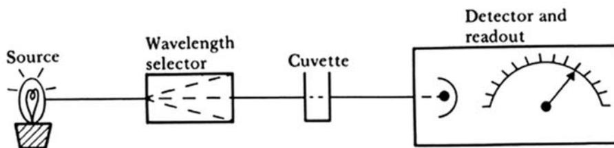
**Figure 11.1** Block diagram of a spectrophotometer (Based on R. J. Henry, D. C. Cannon, and J. W. Winkelman, eds., *Clinical Chemistry*, 2nd ed. Hagerstown, MD: Harper & Row, 1974.)
