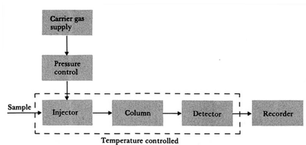
Figure 11.7 Block diagram of a gas-liquid chromatograph (GLC)
