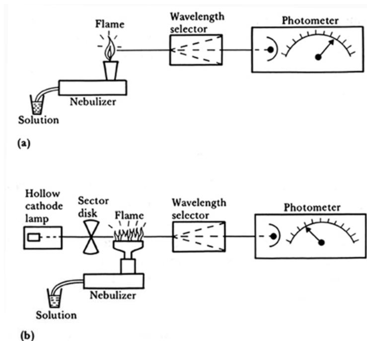
**Figure 11.2** Block diagram of instruments for (a) flame emission and (b) flame absorption. (Based on R. J. Henry, D. C. Cannon, and J. W. Winkelman, eds., *Clinical Chemistry*, 2nd ed. Hagerstown, MD: Harper & Row, 1974.)
