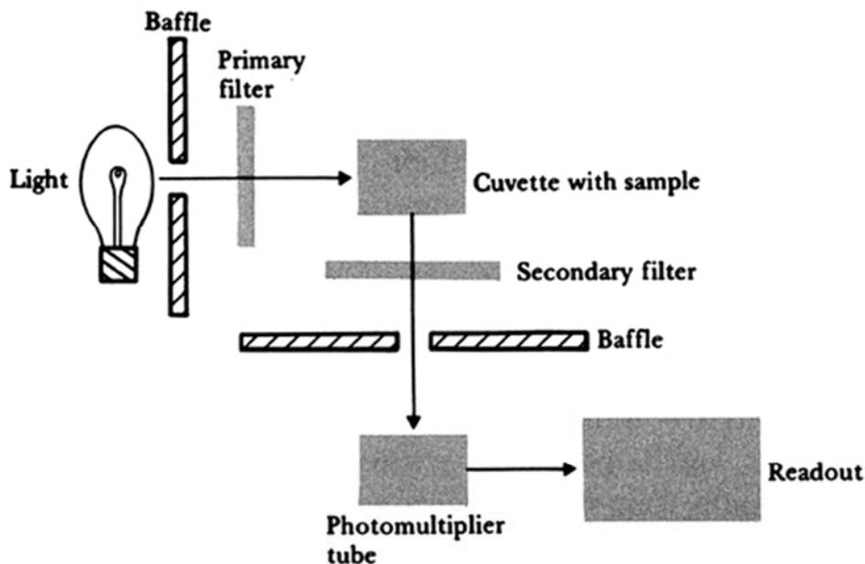
**Figure 11.3 Block diagram of a fluorometer** (Based on R. Hicks, J. R. Schenken, and M. A. Steinrauf, *Laboratory Instrumentation*. Hagerstown, MD: Harper & Row, 1974. Used with permission of C. A. McWhorter.)
