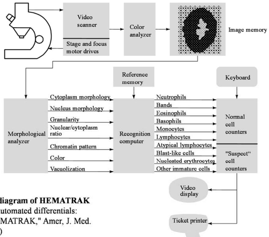
**Figure 11.14 Block diagram of HEMATRAK**
