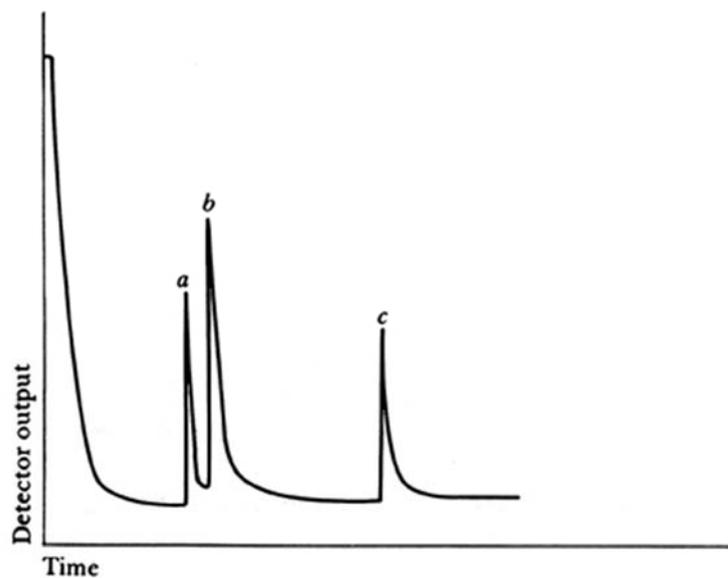
**Figure 11.8** Example of a GLC recording for the analysis of blood levels of phenobarbital (peak *a*) and phenytoin (peak *c*). Peak *b* corresponds to the level of heptabarbital (the internal standard).
